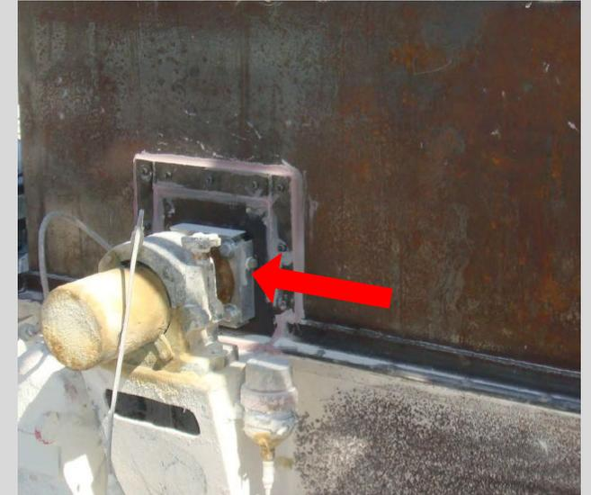
**After:** Inpro/Seal Air Mizer CEMA shaft seal installed
