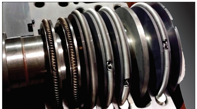
Process steam turbine gland box with Sentinel Floating Brush Seals in the first and second positions (furthest left) and conventional carbon rings in the four remaining positions.
