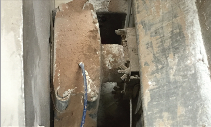
Leaking pancake mix covers the mixer, increasing maintenance costs and equipment downtime.
