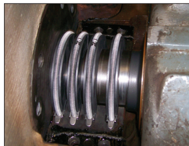
Typical gland box outfitted with conventional carbon rings
