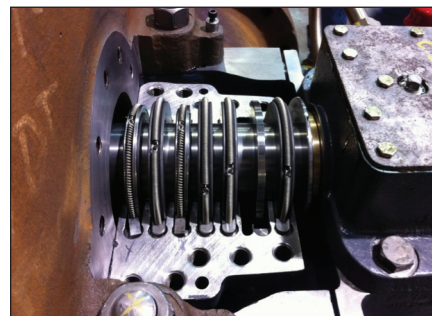
Gland box upgrade with two Sentinel Floating Brush Seals
